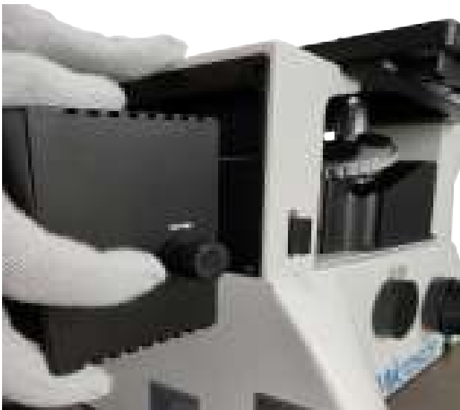
Lamp House Installation
